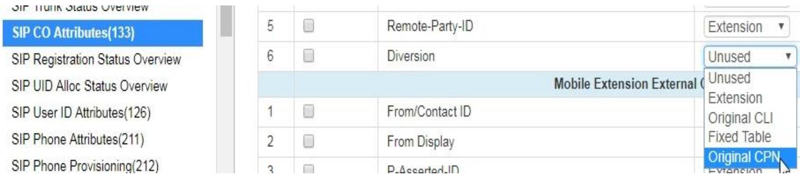
The screenshot shows a configuration interface for SIP attributes. On the left, a sidebar lists various SIP-related sections, with 'SIP CO Attributes(133)' selected. The main area displays a table of attributes. The 'Diversion' attribute is highlighted, and a dropdown menu is open, showing options: 'Unused', 'Extension', 'Original CLI', 'Fixed Table', and 'Original CPN'. The 'Original CPN' option is currently selected.
